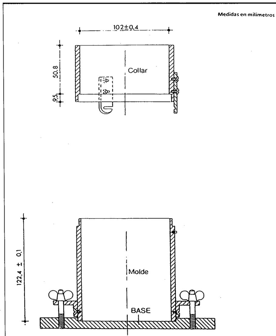
FIGURA 1. Molde Proctor normal
